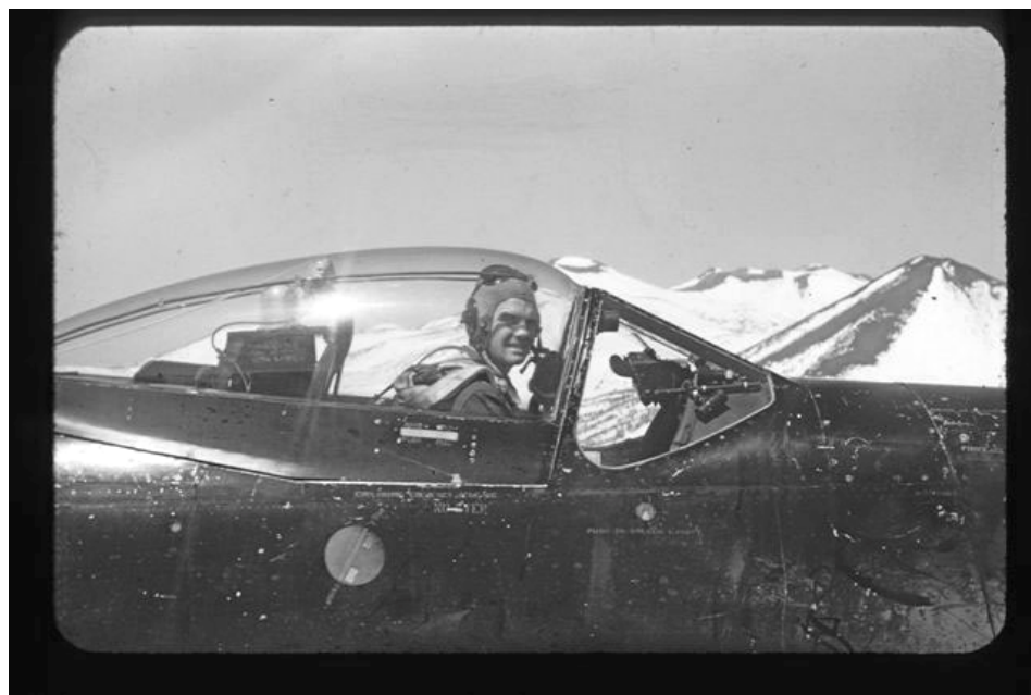
35. In the Korean War Charlie flew the F-82G "Twin Mustang," an all-weather fighter-bomber with the pilot in the left cockpit and the radar observer in the right cockpit. This photo of Charlie was taken in flight over Japan by his radar observer.
